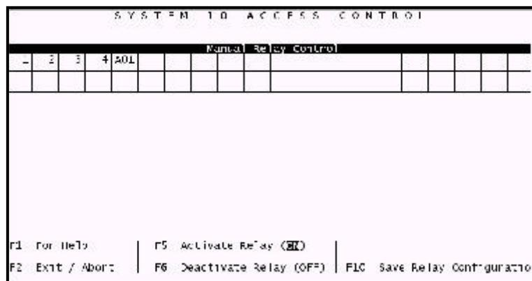
Figure 5.2 - Manual Relay Screen
